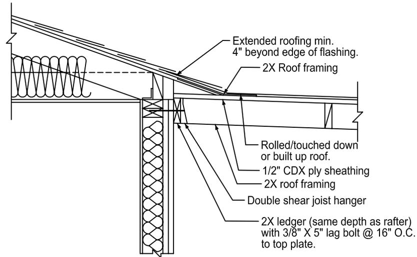
Figure 8 / Typical Ledger Details
